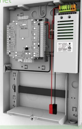
The 12/24V 2A AC/DC Power supply unit is available in either a plastic or metal cabinet. The cabinet can house both the 12/24V 2A AC/DC PSU and a Net2 ACU with the option to accommodate a 12V/7Ah back up battery if desired. A tamper switch is also installed which registers an alarm if the lid is opened when connected to an ACU.
